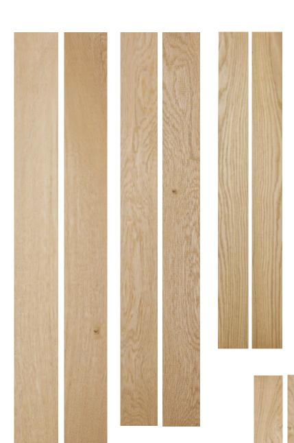
For all grades, the letter X indicates the presence of sound sapwood less than two thirds of the thickness, and XX if it is present on both faces.
