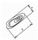
Knot sizes are measured as the average of their largest and smallest diameters
